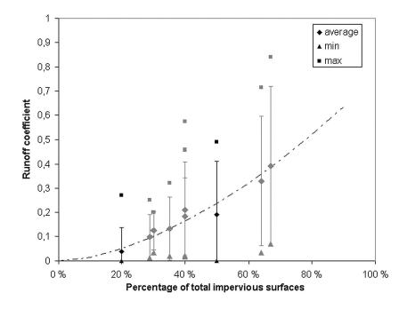
Figure 2. Event runoff coefficients as a function of total catchment imperviousness (from Metsäranta et al. 2005)
